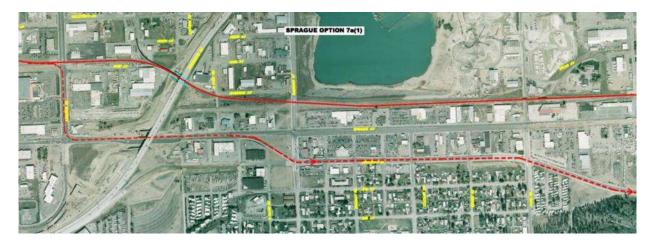
Option #7 was subsequently modified to transition from Sprague to Appleway at Thierman to avoid the I-90 interchange. The modified option is referred to as 7a(2), shown below.
